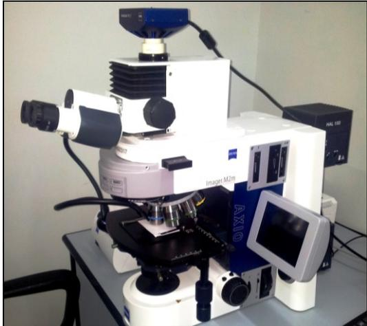
A photograph of a Zeiss Axio-Imager M2m microscope. It is a white and blue compound microscope with a digital camera mounted on top. The camera is connected to a computer monitor and a keyboard. The microscope is sitting on a black table.  |
